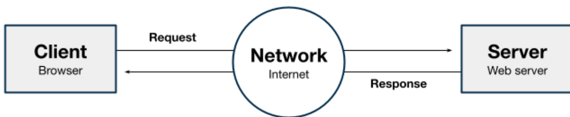
Figure 1.14, HTTP communication process.
